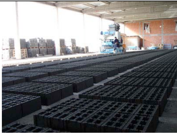
Hollow blocks production
